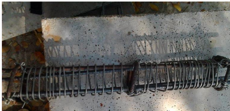
Figure 2.4: Continuous spiral reinforcement
