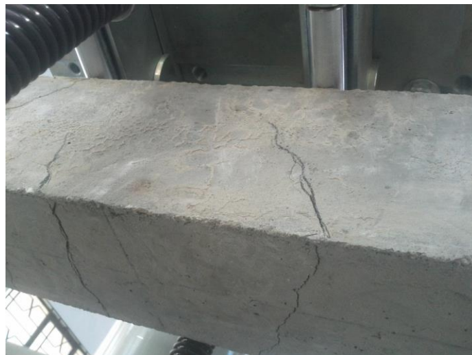
Figure 3.2: Formation of cracks in beam
